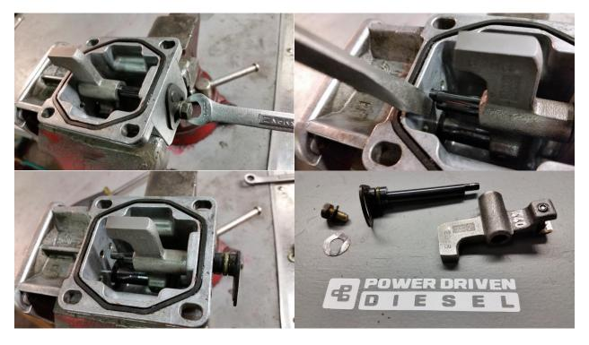
7. Next, remove the AFC foot by removing (1) 10mm bolt and using a screw driver to pry the guide rod assembly free from the AFC housing.
