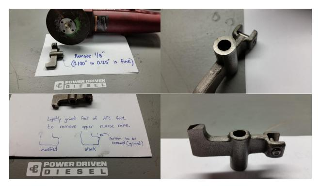
8. Using a grinder or cut-off wheel, remove 1/8" (0.125") from the guide barrel of the AFC foot, for maximum AFC foot travel a minimum 0.100" must be removed. Optional: lightly grind the face of the AFC foot to remove the reverse/negative rake on the upper portion of the foot. The dark portion of the foot face in the picture is left stock, only the upper half is lightly ground flat to remove the upper reverse rake.
