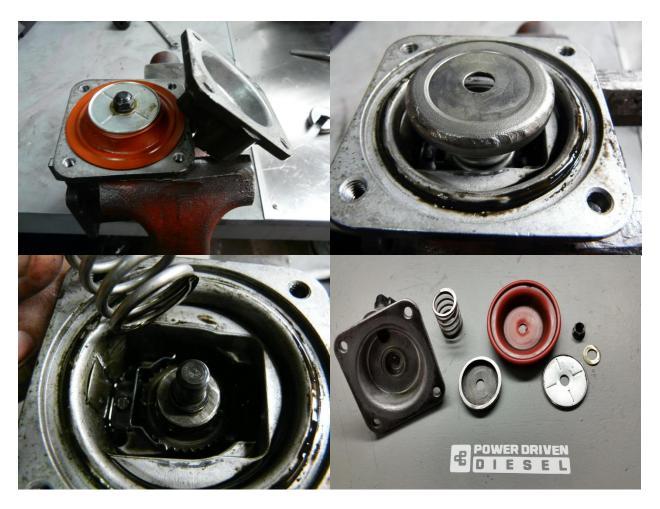
6. Under the AFC back cover is a red rubber-like diaphragm. Remove the 10mm nut, small washer, large washer, diaphragm, inner cupped washer, and stock AFC spring.
