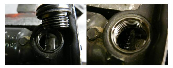
10. Remove the 5/16" or 8mm allen socket plug on the top of the AFC to gain access to the star wheel. If this plug has never been removed, it will be pretty tight and may require a vise to hold the AFC when breaking it loose. (It's regular standard thread: righty-tighty, lefty-loosey)
