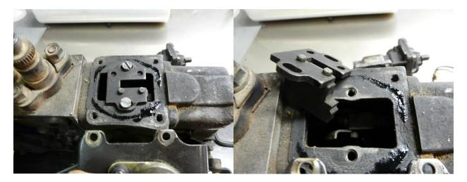
4. Remove the fuel plate being careful to not drop screws or washers into the open governor housing. If the fuel plate is left installed, it will limit injection pump fueling long before the AFC reaches full travel. This AFC Max Travel Kit is designed to provide full AFC foot travel, therefore fuel plate removal is recommended. It's advisable to use a magnet when removing the screws.
