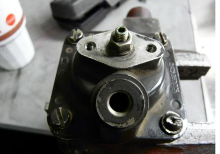
flat-standard screws and grinding a slot in (1) tamper-proof screw and then removing screw. Also grind a slot in the tamper-proof screw on the small pre-boost fuel cover and remove the cover. A sharp chisel can also be used to make a slot. Pliers or vice grips are another method for tamper screw removal.
