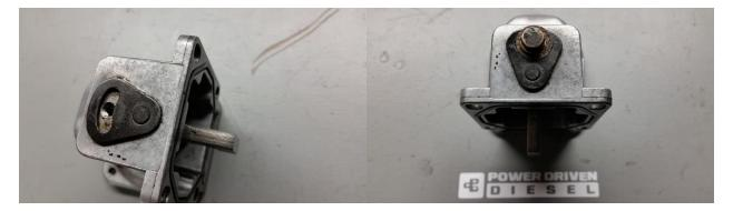
9. Clean and re-install the AFC foot by installing the guide rod into the housing and through the AFC foot/barrel. Install the AFC foot facing rearward towards the AFC diaphragm like the stock orientation pictured in step 6 above. Note the orientation of the guide rod tab vs. bolt so the AFC foot height can be reset to the stock setting, it's typically not fussy but if the old orientation wasn't noted, start with the slotted tab centered over the bolt hole as pictured.
