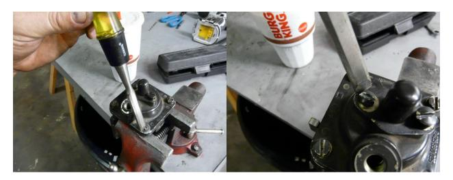
5. Take the AFC to a suitable working location (work bench). Remove AFC cover by removing (3)
